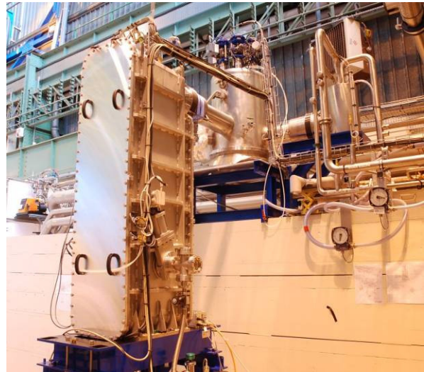
Figure 1: Cryomodule inside the test stand, connected to the valves box. RF coupler is below, hidden by the support frame.
