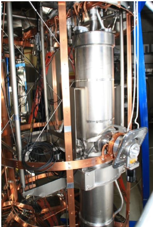
Figure 8: One prototype cavity installed in the cryostat before shield cooling MLI and magnetic shielding were added.
