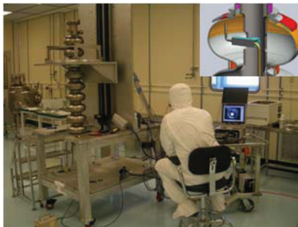
Figure 1: Cavity surface inspection station. Presently, only up/down control is computer controlled. In the inset shown is a design drawing of the inspection with a videoscope.
