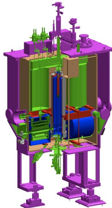
Figure 5. Isometric sectional view of the rebuncher cryomodule.
