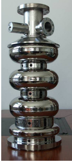
Figure 5: Large grain niobium 3.5-cell cavity made by PKU.
