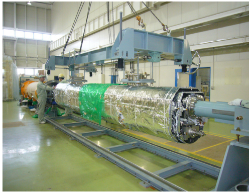
Figure 3: Insertion of an assembled cold mass into a vacuum vessel.
