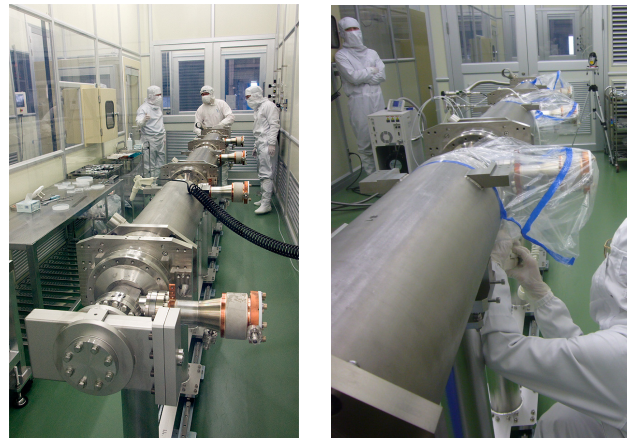
Figure 1: String assembly in a class-10 clean room (left) and vacuum leak-check in a class-1000 clean room (right).
