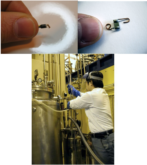
Figure 3: Commercial and ANL in-house germanium resistance thermometers (top) and 2 nd sound testing in a 6" He dewar (bottom).
