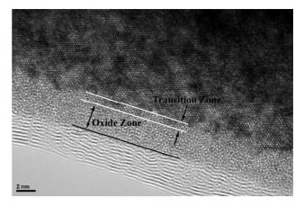
Figure 7: Atomically resolved TEM cross-section image of an BCP treated Nb sample that shows more surface area. The oxide layer and a possible transition zone between the  $Nb_2O_5$  and the bulk Nb is indicated.
