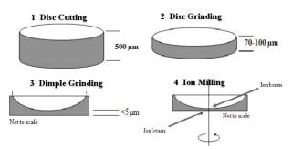
Figure 3: Illustration on the steps for getting final Nb TEM cross-section samples after the steps shown in Figure 2.
