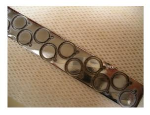
Figure 6: FG samples ( $\emptyset$  8 mm) cut by water-jet; Nb sheet (140 x 10 mm) was electropolished first.
