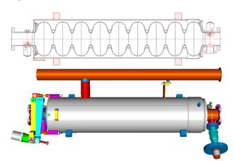
Figure 1: SRF cavity in LHe tank with auxiliaries.
