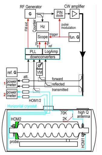
Figure 2: Superconducting cavity CW test in horizontal test cryostat.
