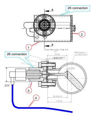
Figure 3: HOM coupler with a new feedthrough (JLAB design), with temperature sensors positions.
