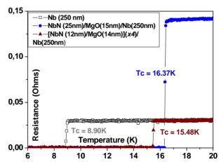
Figure 1: Resistive transition of an Nb film covered or not by a NbN/MgO multilayer
