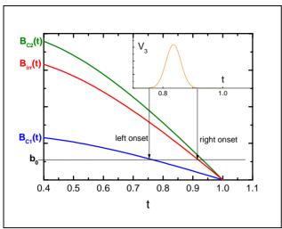
Figure 4: principle of third harmonic analysis (see text for details). t =T/Tc
