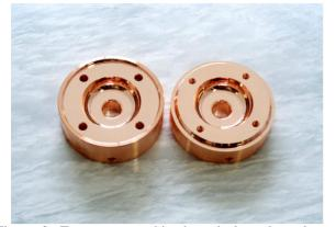
Figure 2: Two parts machined vertical to the axis are assembled to make a cavity. The inside surface is to be covered with  $MgB_2$  films.
