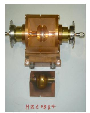
Figure 7: Host cavity for the measurement of a quadrant.
