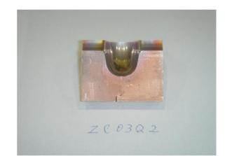
Figure 4: A quadrant cut from the assembled cavity. The contact plane can be seen along the equator line and the cross section. Here, the inner surface is covered by YSZ.
