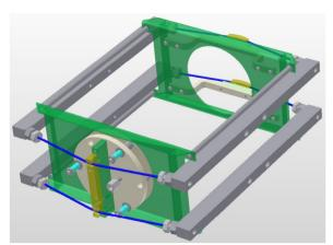
Figure 3: The ANL Intensity Upgrade pneumatic slow tuner: bellows (light gray), wire rope (blue), and bars which bolt to beam ports (dark gray).
