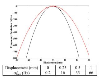
Figure 2: Quarter wave cavity resonator frequency's dependence on center conductor displacement (Top). The black data is for displacements along the beam line, the red data is for displacements perpendicular to the beam line. The table gives the expected peak-to-peak detuning amplitude for several displacements of the center conductor along the beam axis (Bottom).
