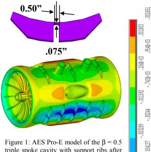
Figure 1: AES Pro-E model of the  $\beta = 0.5$  triple spoke cavity with support ribs after modifications. Displacements are in inches.
