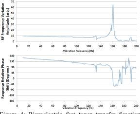
Figure 4: Piezoelectric fast tuner transfer function with a 169 MHz halfwave cavity.
