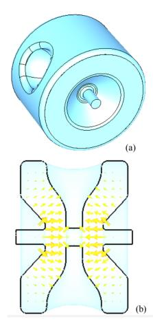
Figure 6: (a) Spoke resonator designed in CST Microwave studio (b) Electric field profile in the spoke resonator.
