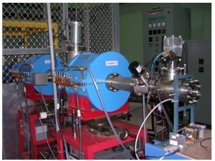
Figure 3: LEBT test bench at BARC.
