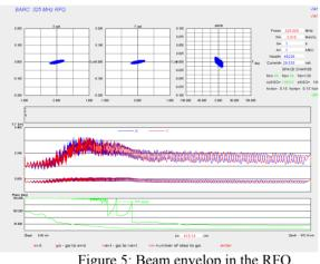
Figure 5: Beam envelop in the RFQ.
