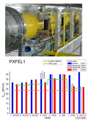
Figure 5: (top) Prototype XFEL cryomodule at FLASH, and (bottom) field gradient distribution [22].
