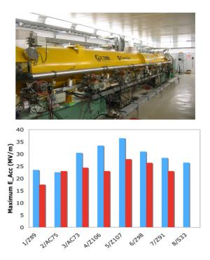
Figure 6: (top) Cromodule-1 at NML, and (bottom) the field gradient distribution (right) compared with individual test in horizontal position (left) [23].
