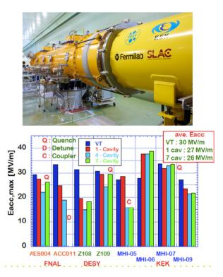
Figure 7: (top) S1-global cryomodule installed at STF, and (bottom) the gradient distribution in cavity-string operation (right three) compared with the result from their individual vertical test (most left) [24, 27, 28].
