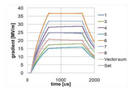
Figure 8: LLRF control to compensate the Lorentz force detuning, and the vector sum stability in S1-Global cavity-string test.
