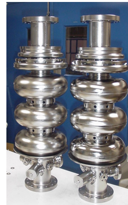
Figure 11: SRF gun cavities for ELBE.
