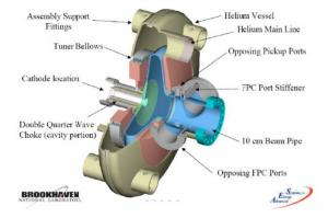
Figure 4: 704 MHz elliptical SRF gun.
