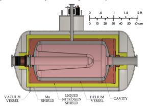
Figure 5: 112 MHz electron gun cryomodule.
