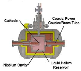
Figure 6: 500 MHz NPS QWR gun.
