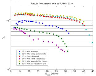
Figure 3: Results of  $1\frac{1}{2}$  cell gun cavity vertical testing at Jefferson Lab.
