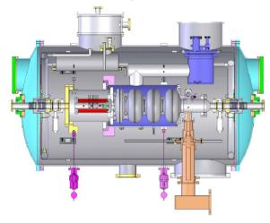
Figure 1: DC-SRF gun at Peking University.
