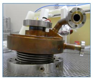
Figure 5: New cathode cooler.
