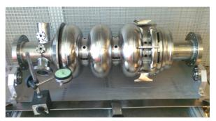
Figure 2: The status of the cavity fabrication.
