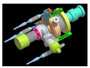
Figure 4: 3D model of the cathode cooler.
