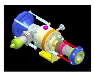
Figure 9: Completed solenoid part on the beam pipe.
