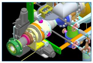
Figure 10: Solenoid with two step motors.
