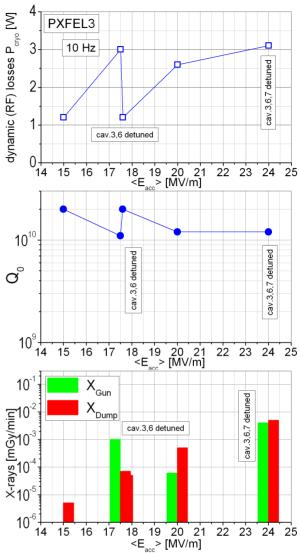
Figure 9: Module PXFEL3 dynamic cryogenic losses, module  $Q_0$  and gamma radiation.
