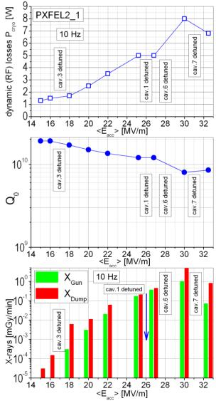
Figure 5: Module PXFEL2\_1dynamic cryogenic losses, module  $Q_0$  and gamma radiation.
