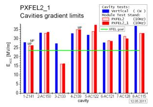
Figure 2: Module PXFEL2\_1 cavities gradient limits.
