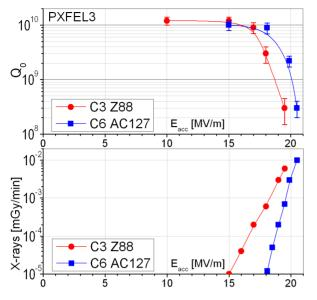
Figure 10: Module PXFEL3 cavities 3 and 6 retested in the horizontal cryostat after module disassembly.
