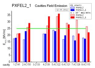
Figure 3: Module PXFEL2\_1 cavities Field Emission onsets compared to maximum gradient.
