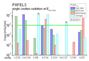
Figure 8: Module PXFEL3 cavities gamma radiation (cyan – single cavities retested after disassembly: H – horizontal cryostat pulsed test, others – vertical cryostat CW test).
