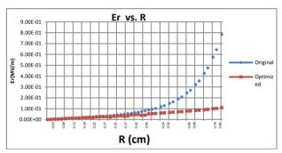
Figure 3: Transverse field distribution on cathode before(♠) and after(■) optimization.
