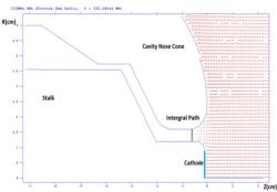
Figure 2: Field distribution near cathode surface and nose cone.
