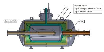
Figure 1: The layout of 112MHz electron gun with the new cathode stalk and fundamental power coupler.
