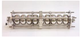
Figure 1: IHEP-01 low-loss large grain 9-cell cavity.
