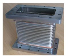
Figure 2: Rectangular stainless steel bellow (100 mm length) as part of the rf waveguide transition (WR 284) for the injector upgrade module (before copper plating).
