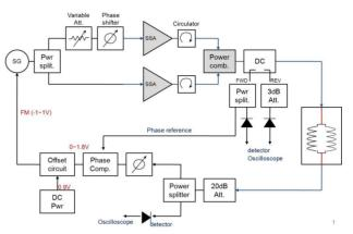
Figure 7: RF System setup for the vertical test.
