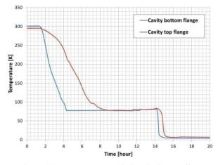
Figure 14: Temperature variation during cooling.
