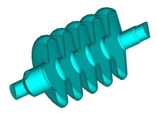
Figure 3: Five-cell prototype cavity.
