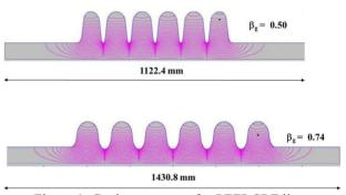
Figure 1: Cavity geometry for PEFP SRF linac.
