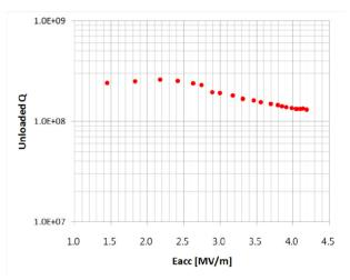
Figure 16: Q0 vs. Eacc for the prototype cavity.
