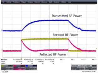
Figure 15: RF pulse waveform during the vertical test.
