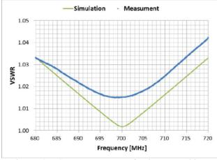
Figure 10: VSWR measurement for the RF combiner.
