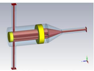
Figure 8: Split coaxial type RF combiner.
