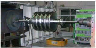
Figure 4: Electron-beam welding of five-cell cavity.
