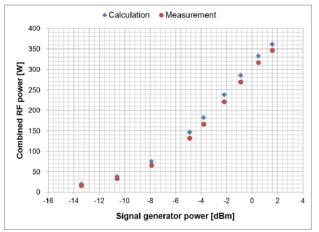
Figure 11: High power performance of the RF combiner.
