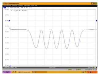
Figure 6: Field distribution after field flatness tuning.
