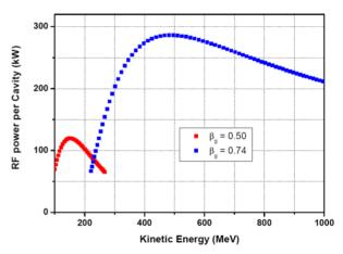
Figure 2: RF power requirement for each cavity.
