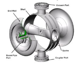
Figure 4: Exploded view of SSR0.
