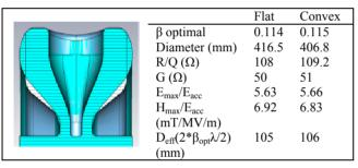
Figure 2: Comparison between the original and convex RF design of SSR0. The final design is highlighted in blue. The table to the right shows that the main RF parameters were virtually unaffected.
