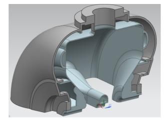
Figure 10: SSR1 with the new helium vessel design for project X. Both walls of the helium vessel (in gray color) are coupled to the end walls of the cavity (in light blue) by means of a bolted connection.
