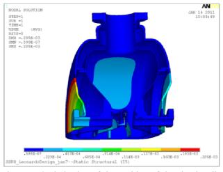
Figure 5: Optimization of the position of the circular rib to minimize df/dP. The left beam pipe is connected with bellows to the helium vessel, the right one is welded. This analysis produced a result of 5 Hz/torr.
