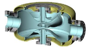
Figure 9: Design of the jacketed SSR0. The Niobium components are shown in light blue color, The stainless steel parts are instead shown in yellow and gray colors.
