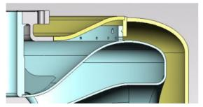
Figure 6: Details of the bolted connection between the end-wall and the helium vessel of SSR0. The end-wall shown is the one without a bellows.
