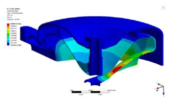
Figure 8: Residual plastic deformation (under 100  $\mu$ m) after the application of 2.5 bar of pressure and relaxation.
