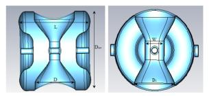
Figure 11: Cross-section of SSR2. L - cavity length, D - spoke diameter, W - spoke width,  $D_{cav} - cavity diameter$ .
