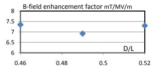
Figure 3: Magnetic field enhancement factor vs. D/L ratio for SSR0 with convex end-walls.
