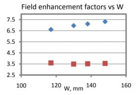
Figure 13: Field enhancement factors vs. W. Red  $E_{peak}/E_{acc}$ , blue  $B_{peak}/E_{acc}$  (mT/<sup>MV</sup>/<sub>m</sub>).
