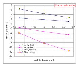
Figure 19: cHWR at different external pressure and beam pipe constrains.
