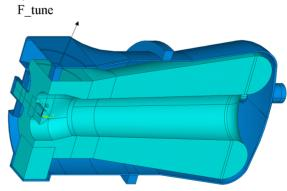
Figure 13: cHWR tune simulation model.
