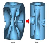
Figure 6: SSR0 geometry transformation into HWR.
