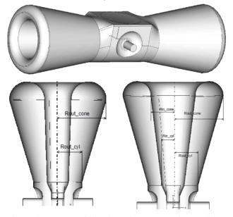
Figure 1: HWR with enlarged outer conductor dome diameter.
