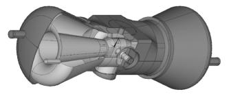
Figure 10: cHWR with helium vessel.
