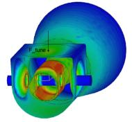
Figure 5: cHWR simulation tune model.
