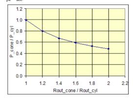
Figure 2: Power dissipation in conical HWR relative to cylindrical shape.
