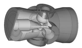
Figure 18: cHWR with helium vessel simulation model.
