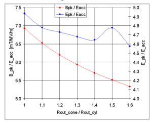
Figure 8: Peak magnetic and electrical fields in cHWR.
