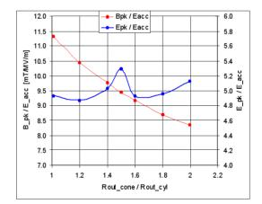
Figure 3: Peak magnetic and electrical fields in conical cavity.
