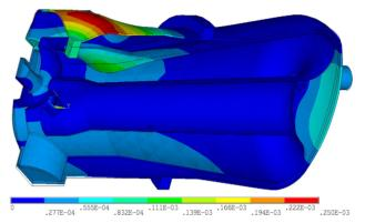
Figure 12: cHWR under external pressure with helium vessel.
