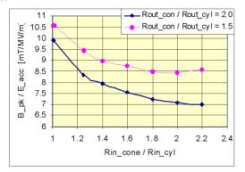
Figure 4: Peak magnetic field in conical cavity with enlarged central electrode dome diameter.
