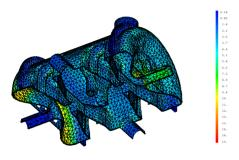
Figure 4: Von Mises stress distribution, unit: MPa
