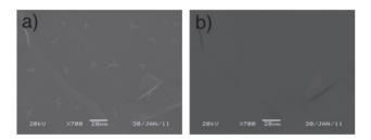
Figure 7: Secondary electron (a) and backscattered electrons (b) images of the same area covered with precipitates on the 130-7 hot spot cutout.
