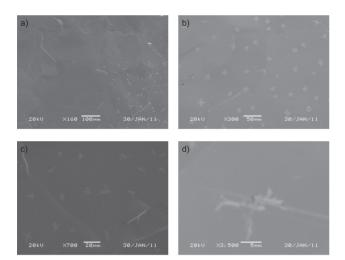
Figure 5: SEM secondary electron images of the dendritic objects found on the 130-7 hot spot cutout.
