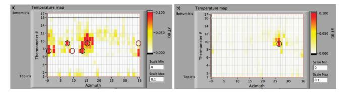
Figure 2: Temperature maps at  $H_{peak} = 160 mT$  right before (a) and after (b) quench. Locations from where the samples were extracted are marked with black circles for hot spots and quench location, and brown circles for sites with negligible RF losses (cold spots).
