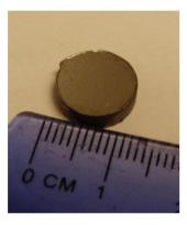
Figure 3: Typical cutout sample extracted from cavity walls. A ruler is shown for comparison.
