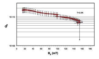
Figure 1: The quality factor  $Q_0$  of the cavity plotted against the peak surface magnetic field  $H_{peak}$  as measured during the RF test.
