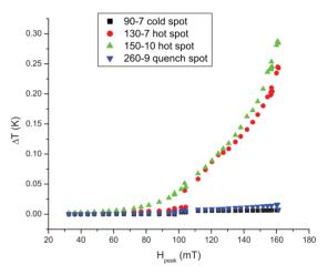
Figure 4: Temperature sensor readings versus peak magnetic field for two hot spots, one cold spot, and a quench site prior to the quench.
