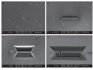
Figure 8: Steps in FIB preparation of site-specific sample for TEM: (a) area of carbon deposition marked by a ; (b) after carbon deposition; (c) after rough milling; (d) membrane ready to be extracted by omniprobe.
