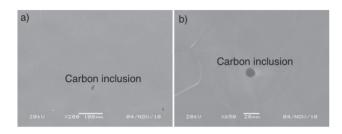
Figure 10: SEM images of the carbon inclusions found on the surface of the cutout from the quench site.
