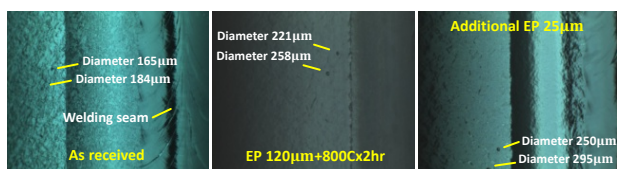
Figure 6: The geometrical evolution of one defect in 9-cell cavity TB9RI019 with chemical treatment in cavity.
