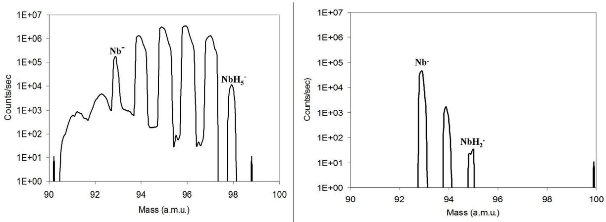
FIGURE 1: SIMS mass spectra showing difference in H between (left) non-heat treated and (right) heat treated sample.
