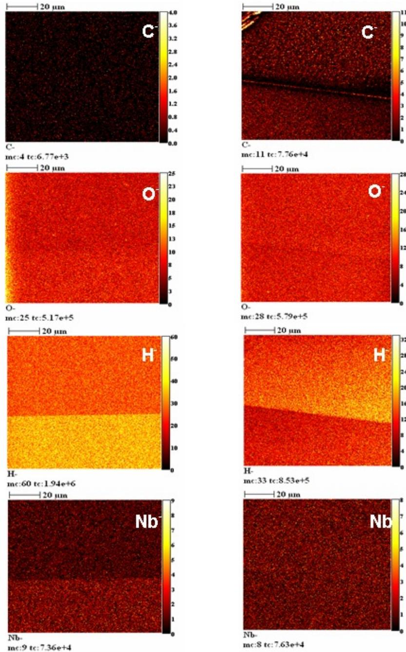
FIGURE 5: Grain boundary ion images of control (left column) and heat treated (right column) bicrystal samples.
