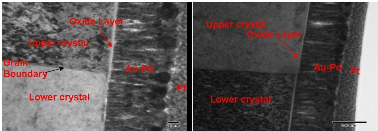
FIGURE 3: TEM micrographs of control (left) and heat treated (right) bicrystal samples.
