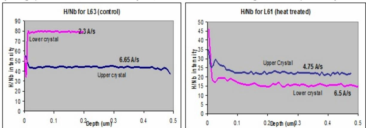
FIGURE 4: H/Nb intensities for control (left) and heat treated (right) samples extracted from the dynamic SIMS measurements.
