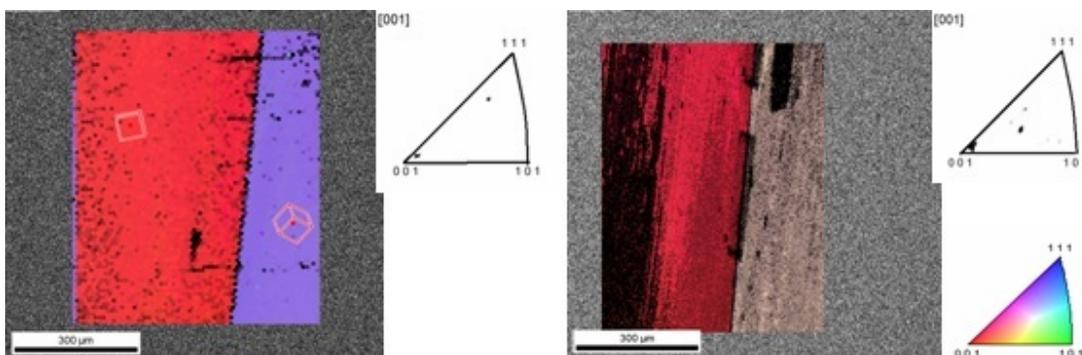
FIGURE 2: EBSD results for control (left) and heat treated (right) bicrystal samples. Color coding similar for both samples.
