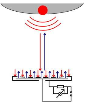
Figure 3: Schematic drawing of the second sound detection with an OST. He-I (red) is "blocked" by the porous membrane and exerts pressure, while the counterflow of He-II may pass the membrane easily.
