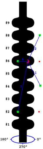
Figure 6: Plot of a 9-cell cavity with the positions of the OSTs marked with squares. The green OSTs are the used ones for the determination of the quench location and the blue lines point to the quench location as calculated with the MATLAB code.
