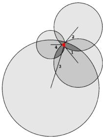
Figure 5: Spheres including the distance propagated by second sound. The intersecting volume is the most likely quench location.
