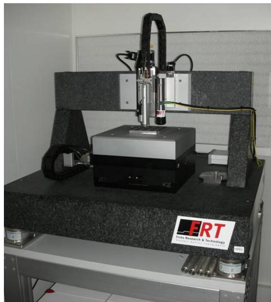
Figure 3: Optical profilometer with AFM.
