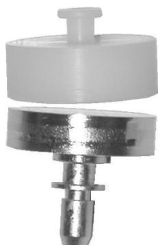
Figure 4: LG Nb sample with the protection cap.
