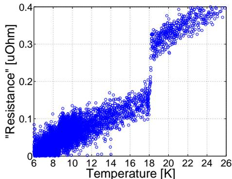
Figure 8: 4-wire measurement of the  $\text{Nb}_3\text{Sn}$  sample indicates a critical temperature of  $\sim 18.1 \text{ K}$
