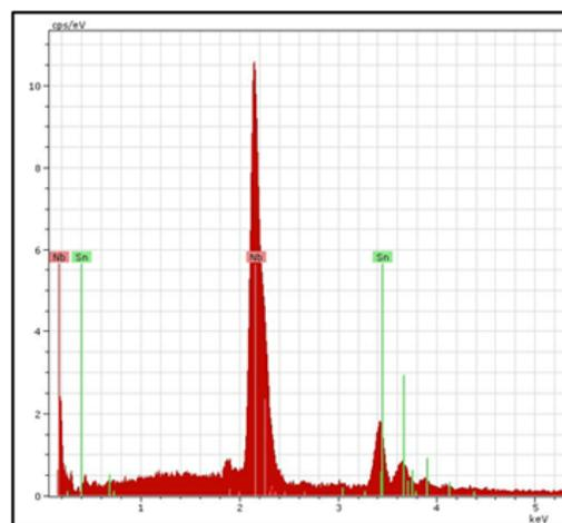
Figure 5: EDX spectrum of Nb<sub>3</sub>Sn sample indicates composition  $\sim 24.2$  atm%Sn.
