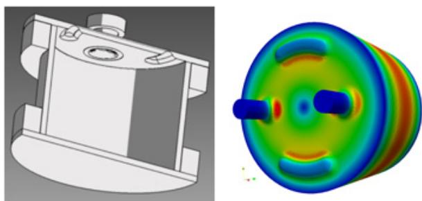
Figure 11: CAD (left) and CST (right) models of the Cornell TE Pillbox Cavity.
