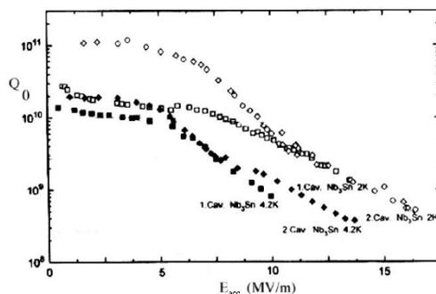
Figure 1: The best results obtained at University of Wuppertal for 1.5 GHz cavities vapor-diffusion coated with Nb<sub>3</sub>Sn. From [4].
