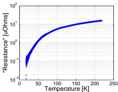
Figure 9: Resistance of sample versus temperature shows that minimal RRR degradation occurred during coating process.
