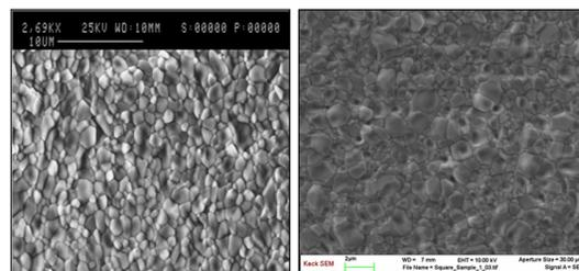
Figure 4: SEM images of Nb<sub>3</sub>Sn produced at Wuppertal in 1996 (left) and at Cornell in 2011 (right).
