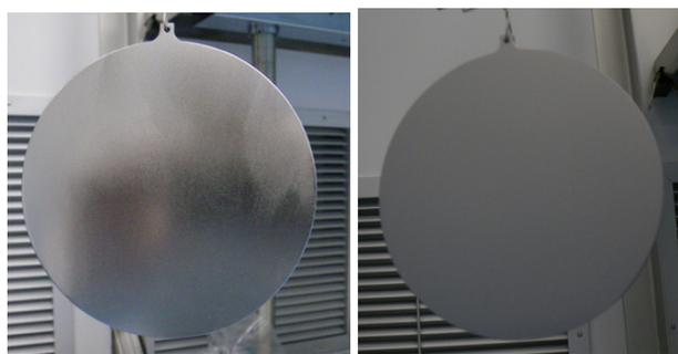
Figure 10: Pictures of pillbox cavity bottom plate before (left) and after (right) Nb<sub>3</sub>Sn coating.
