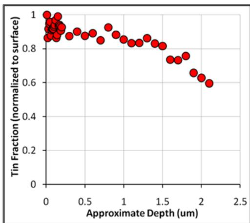
Figure 7: Alternately sputtering sample and performing XPS scans shows composition versus depth.
