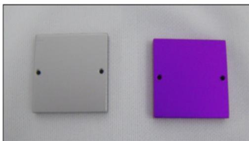
Figure 3: Nb<sub>3</sub>Sn-coated sample (left) and an identical sample after anodization in NH<sub>4</sub>OH at 75 V (right). The pink-purple color indicates Nb<sub>3</sub>Sn phase on surface.
