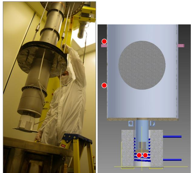
Figure 2: The Nb<sub>3</sub>Sn coating chamber being inserted into the UHV furnace (left) and a cross section (right) showing the tin crucible surrounded by the heater and the substrate suspended above. The red circles represent thermocouples for temperature monitoring.
