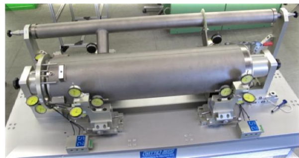
Figure 6: control device with Helium tank installed for quality control.
