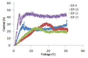
Figure 7: The Cavity I-V curves from the different cathode shapes in EP experiments (EP-9: ball cathode; EP-10: thin bar cathode; EP-11: thick bar cathode; EP-12: wheel cathode 3).
