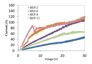
Figure 2: The cavity I-V curves from the different cathode shapes in BEP experiment series 1 (BEP-2: thin bar cathode; BEP-6: ellipsoid cathode; BEP-8: ball cathode; BEP-13: wheel cathode 3; BEP-14: thick bar cathode).
