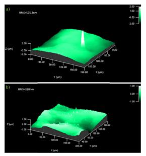
Figure 13: Typical Profilometer images of the surfaces of the button samples from the demountable cavity treated by EP process with a scanned area of  $(200 \times 200)$  µm2. a) Sample 1; b) Sample 3.
