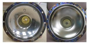
Figure 10: The CCD pictures of single cell cavity treated by BEP process with the wheel cathode 3. Left one is the upper half cell; right one is the lower half cell.
