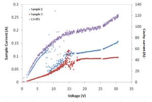
Figure 4: The I-V curves in the BEP experiment using the ball shape cathode.
