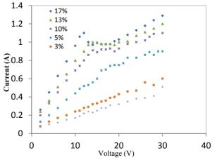
Figure 3: The I-V curves obtained from small sample experiments with different cathode area during BEP. The percentages shown in the figure are the surface area ratios between cathode and anode.
