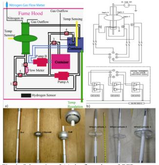
Fig. 1: Schematics of (a) the flow chart of BEP system and (b) the data acquisition system of the vertical BEP system for Nb SRF single cell cavities and the cathodes used in this study.
