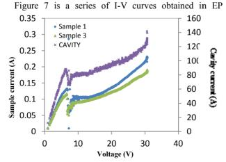
Figure 6: The I-V curves in BEP experiment using the wheel cathode 3.
