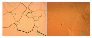
Figure 12: The MOM pictures of button samples from the demountable cavity treated by BEP process with the wheel cathode 3. Left one is measured on sample 1; right one is measured on sample 3.
