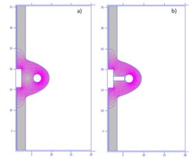
Figure 5: The simulated electric field distributions in the cavity with wheel cathode 3.
