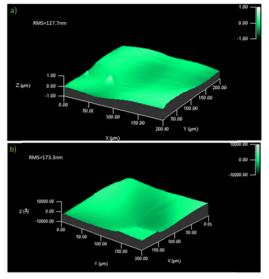
Figure 14: Typical Profilometer images of the surfaces of the button samples from the demountable cavity treated by BEP process with a scanned area of  $(200 \times 200) \mu m2$ . a) Sample 1; b) Sample 3.
