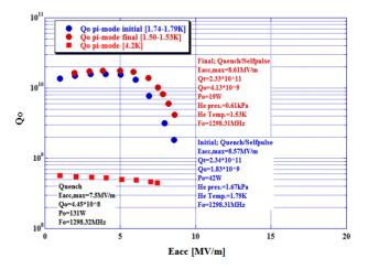
Figure 7: RF test result of the 9-cell cavity. Low current density EP-II (20  $\mu$ m) with N<sub>2</sub> gas flow, rinse with ultrapure water (1.5 hrs), detergent rinse with FM\_20 of 2 % (50 °C, 2 hrs), HPR (10 hrs).
