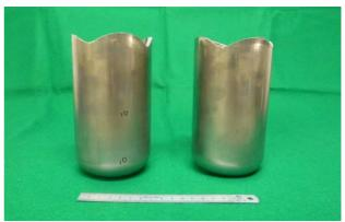
Figure 10: Two long cups formed by deep drawing.
