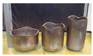
Figure 9: Fabricating process of long cups. (Left: after  $1^{st}$  deep drawing, Center: after  $2^{nd}$  deep drawing, Right: after  $3^{rd}$  deep drawing).
