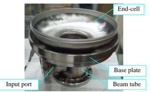
Figure 6: End-group by the side of input port.
