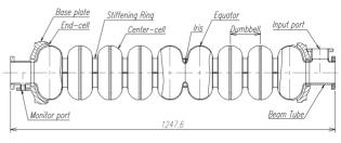
Figure 1: Drawing of 9-cell superconducting cavity without HOM couplers.
