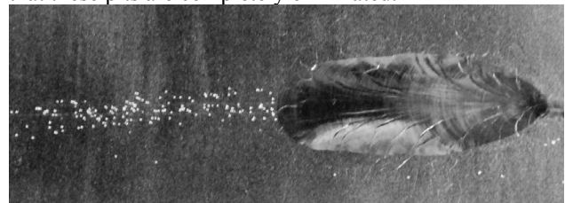
Figure 1: Effect of local electron-beam re-melting. Man-made pits (~200 μm in diameter) are seeded in the central surface region of a niobium sample. Pits are visible in the left area (without re-melting) and are completely eliminated in the right area (with re-melting).
