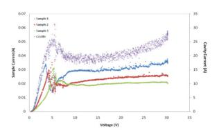
Figure 2: The I V curves in the EP experiment using the ball shape cathode.
