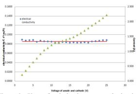
Figure 9: Plots of calculated current and electrical conductivity as a function of voltage.
