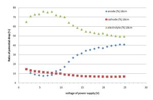
Figure 8: Ratios of potential drops for anode, cathode and electrolyte in BEP process at a distance of 18cm between anode and cathode.
