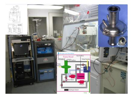
Figure 1: The picture of vertical BEP setup and the demountable cavity.
