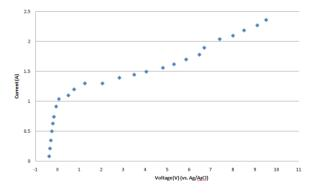
Figure 6: Anode polarization characteristic of Nb in BEP process with reference electrode Ag/AgCl.
