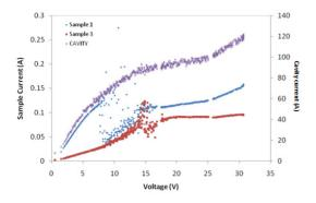
Figure 3: The I-V curves in the BEP experiment employing the ball shape cathode.
