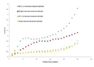
Figure 4: The I-V characteristics at two different distance in small sample experiments.
