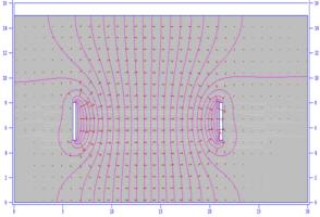
Figure 7: Simulation result of electric field distribution by Possion-Superfish in the small sample experiments.
