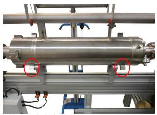
Figure 7: Cavity in a helium tank on new supports.
