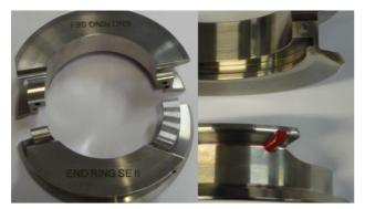
Figure 4: New set of tuning end rings, notice the red marked contact point.
