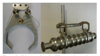
Figure 9: Gripper and cavity lifter carrying a dummy cavity for calibration.
