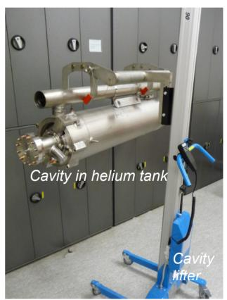
Figure 8: Cavity lifter carrying a cavity in a helium tank.
