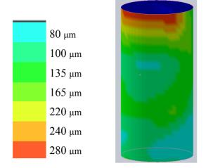
Figure 7: Cavity HWR\_004  $1^{st}$  etch. Desired removal was 135  $\mu$ m.
