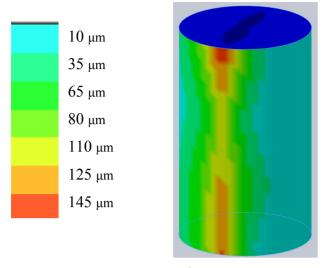
Figure 2: Cavity HWR\_003 1<sup>st</sup> etch. Desired removal: was 100µm.
