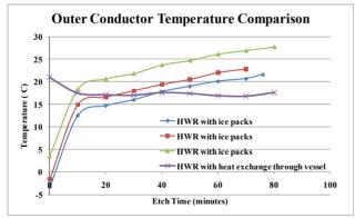
Figure 8: Plot of Outer Conductor surface temperature during etching.
