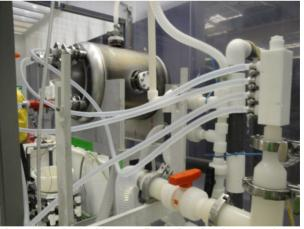
Figure 6: BCP etching configuration for the second set of fixtures using dispensing quills.
