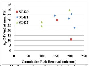
Figure 11:  $E_p$  at maximum field emission levels vs. the cumulative etch removal for three different HWRs.
