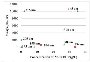
Figure 9: The maximum field emission seen during vertical testing for three different cavities vs. concentration of Nb in BCP at start of etch prior to test.
