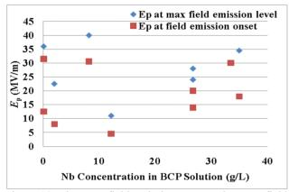
Figure 10: The  $E_p$  at field emission onset and at max field emission level vs. the concentration of Nb in BCP solution at start of etch prior to test.
