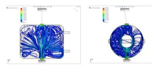
Figure 3: Flow simulation of first chemical etch set-up. BCP enters through bottom port and exits through top RF port.
