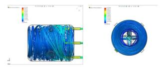
Figure 4: Flow simulation of chosen design. BCP enters through 4 quills and exits through top RF port.
