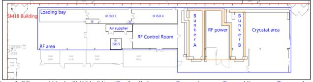
Figure 2: RF area within the SM18 building (①softwall cleanroom, ②preparing area, ③assembling room, ④personal access, ⑤air shower).
