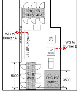
Figure 4 : RF power area, new configuration.
