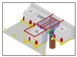
Figure 5 : schematic view of the vertical cryostat area with the clean space.
