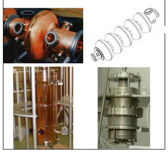
Figure 1: LHC cavity (top left), SPL cavity (top right), HIE Isolde cavity (bottom left), and quadrupole resonator (bottom right).
