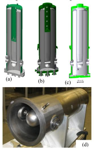
Figure 1: Design evolution of the ReA3 QWR: (a) original RIA QWR prototype; (b) ReA3 production QWR; (c) planned refurbishments for ReA3 (under development); (d) photograph of ReA3 production QWR.
