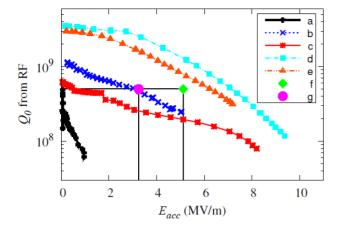
Figure 3: RF performance at 4.3 K of a single cavity (SC246) as it progresses through the R&D leading to the refurbishment. The green diamond (f) indicates the original 4.5 K FRIB goal. The purple circle (g) indicates the 4.5 K ReA3 goal. The curves (a-e) are explained in the text.
