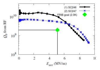
Figure 6: RF tests at 2 K on two refurbished QWRs immersed in a helium bath. The green diamond indicates the FRIB 2 K design goal. Note that  $E_{peak}/E_{acc} = 6.16$ , and  $B_{peak}/E_{acc} = 13.9 \text{ mT/(MV/m)}.$
