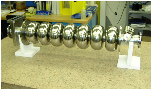
Figure 1: A 12 GeV C100 low-loss shape 7-cell cavity.
