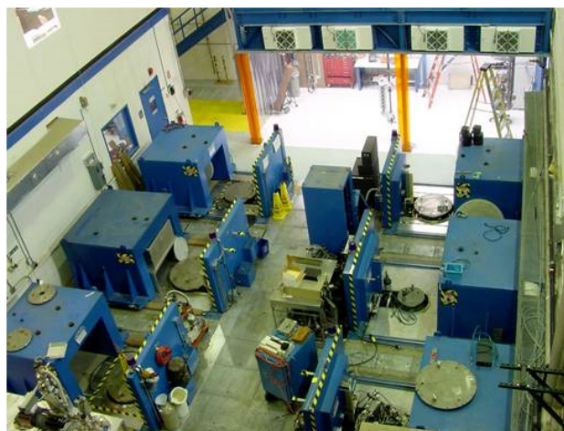
Figure 7: VTA showing six dewars and radiation shields.
