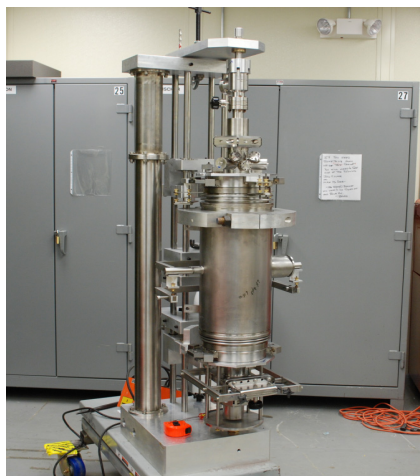
Figure 6: A C100 cavity in the helium vessel tack welding fixture.
