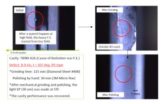
Figure 9: Polishing of pit type defect on the iris.
