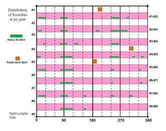
Figure 6: Result of optical inspection of AES-03 at iris.
