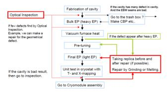
Figure 1: Repair process inclusion for the cavity treatment flow.
