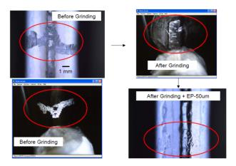
Figure 8: Grind and EP at heavy scratch on iris.
