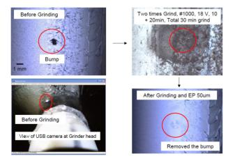
Figure 7: Grind and EP at cell #4 equator.
