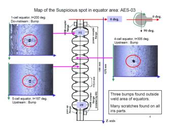
Figure 5: Result of optical inspection of AES-03 at equator.
