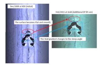
Figure 12: Defect deform by additional EP (85 µm).
