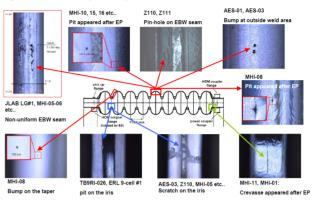
Figure 4: Found geometrical defects by optical inspection.
