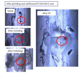
Figure 11: Grinding and EP at JLAB LG#1 cell #5 equator.
