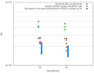
Figure 8: Comparison of  $Q_0$  values for selected LG and fine-grain cavities at DESY, all  $Q_0$  values taken at 15 and 20 MV/m.
