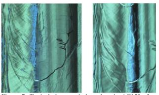
Figure 7: Typical sharp grain-boundary in AC158 after BCP treatment (left), same location after EP with smoothed grain boundary (right).
