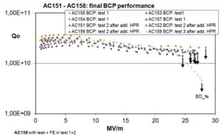
Figure 5:  $Q_0(E)$ -performance after BCP treatment, measured at 2K. All cavities limited by thermalbreakdown; AC158 with strong FE [13].
