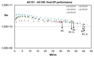
Figure 6:  $Q_0(E)$  performance after EP-treatment, measured at 2K [13].
