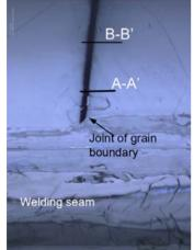
Figure 2: Optical inspection picture of PKU-LG1. B-B' indicates the location of the profile scan in Figure 3 [10].
