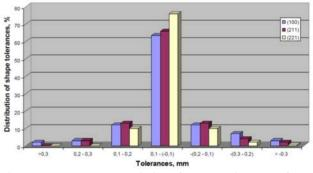
Figure 4: Averaged deviation from the ideal half-cell shape after deep-drawing for different crystal orientations [12].
