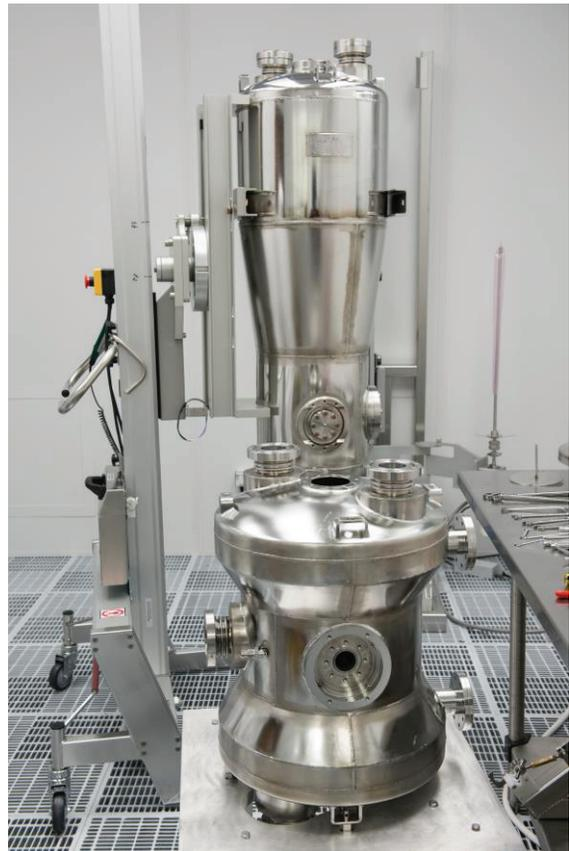
Figure 1: The 72 MHz quarter-wave (back) and the 325 MHz half-wave (front) resonators recently built at ANL.
