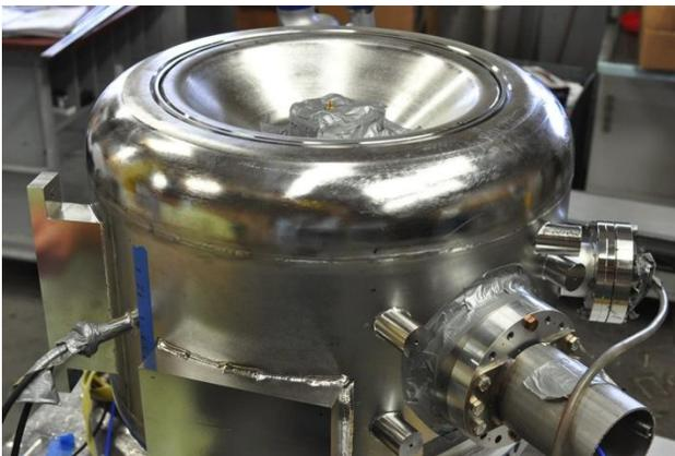
Figure 8 : Final stage of welding operations on SSR1. The transition ring at the top of the picture is not yet welded. Cables and tubes are used to monitor the frequency, temperature and maintain low oxygen count.
