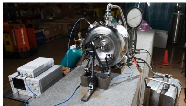
Figure 10: Setup utilized for measuring the sensitivity of the resonator to helium pressure variations. The pressure in the helium circuit was cycled repeatedly using a nitrogen
