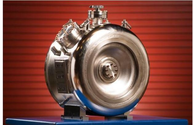
Figure 1 : The first jacketed SSR1 resonator for Project X.
