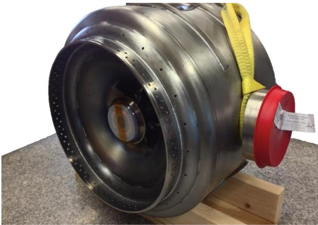
Figure 7 : S107 with the perforated transition ring. The outermost portion of the ring appearing shinier is made of stainless steel.
