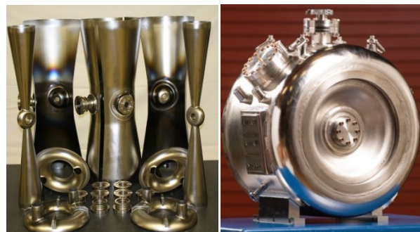
Figure 9: HWR (left) & spoke (right) cavities for PXIE.
