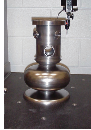
Figure 16: Cavity 1.1 in production at JLab. Here the cavity is only stacked and the first half of the 0.4 \cdot \lambda/2 cell is missing.
