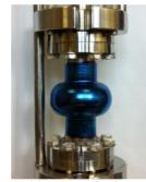
Figure 10: A 6 GHz cavity with a standard external surface (left). The same cavity after the RF test has been anodized only externally (right) and then re-measured. What is important to consider is that such operation is done when keeping the cavity on the stand always under U.H.V.
