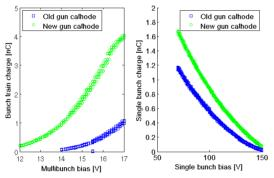
Figure 8: Bunch charges from old, partially depleted linac gun cathode and new cathode installed in September 2013.
