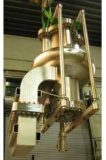
Figure 4: Cavity 4 under test at Cornell University.
