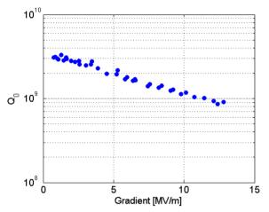
Figure 5:  $Q_0$  as a function of accelerating voltage measured during the vertical test.
