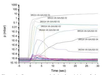
Figure 6: Pressures recorded in the vicinity of the injection straight following the vacuum event in July 2009.
