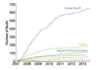
Figure 2: Accumulated faults sorted by technical group. The top three contributing groups are indicated.
