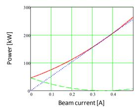
Figure 3: Total amplifier power (red), beam power (blue) and reflected power (green) for three identical CESR cavities in the Diamond storage ring.
