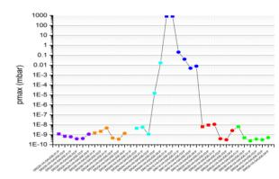
Figure 7: Peak pressures recorded after the July 2009 event. Colours denote different cells, with gauges in the straights (round markers) and arcs (square markers).
