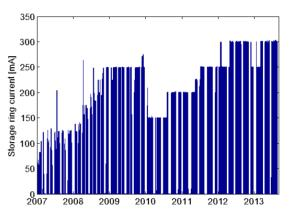
Figure 1: Diamond beam current history. The general envelope shows beam delivered to users, with gaps indicating shutdowns and occasional spikes of test beam in preparation for the next step up.
